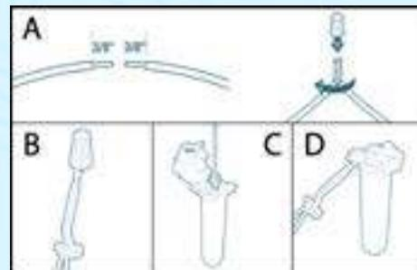
Once you are done with the loop, strip off the ends of the wires and insert both ends into the antenna socket.
