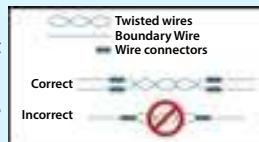
wire nut. Tie a knot 3 to 4 inches from the wire nut (B). Ensure that the wire nut is secure on the wire splice.
